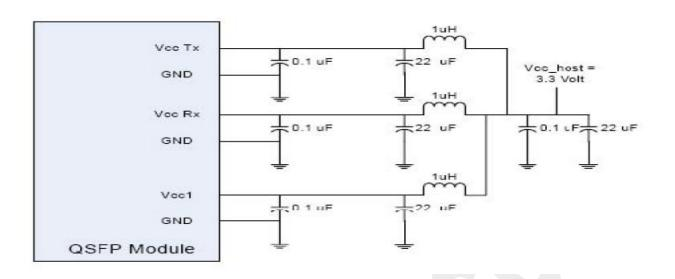
1. GND is the symbol for signal and supply (power) common for QSFP modules. All are common within the QSFP module and all module voltages are referenced to this potential otherwise noted. Connect these directly to the host board signal common ground plane.
